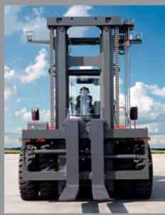
Hydraulic Side-Shift and Fork Positioning with nearly Kissing Forks are a standard feature.
