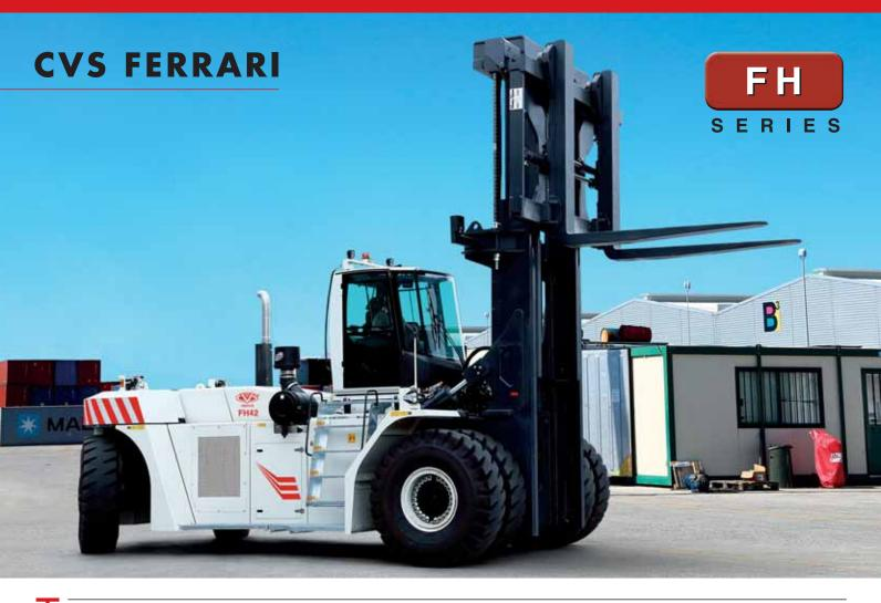
he Driver of a CVS FERRARI Heavy Forklift operates in a solid, safe spacious and comfortable environment. The ARIA cab is equipped with laminated glass, a contoured sun-deflecting front glass and is perfectly sound and temperature insulated. Its visibility and solidity are top class derived from the recessed front pillars and the FOPS upper glass. In its standard configuration it is the most complete and luxurious operator environment in the market.
